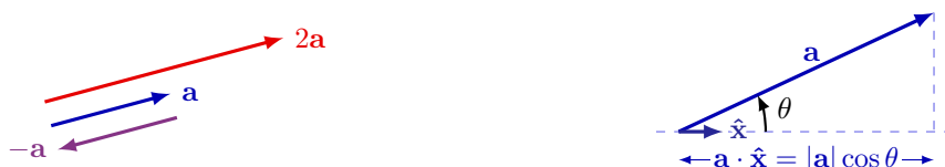
(a) Scalar multiplication b\mathbf{a} of vector \mathbf{a} with scalar b , where b = 2 or -1 . (b) Scalar product x = \mathbf{r} \cdot \hat{\mathbf{x}} is the projection of \mathbf{r} onto the x axis.
