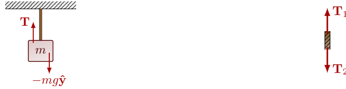
(a) The forces acting on a suspended mass. (b) Piece of string, zoomed in: \mathbf{T}_1 = -\mathbf{T}_2 .
