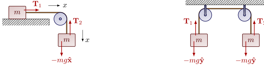
(a) Mass on a frictionless table is pulled by a hanging mass. (b) Atwood machine with two pulleys: Two hanging masses are connecting by a string over two pulleys.
