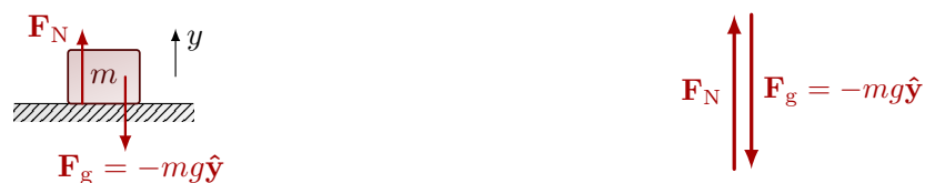
(a) The forces on a mass m at rest: The surface exerts a normal force \mathbf{F}_N , and the Earth a gravitational one, \mathbf{F}_g . (b) The normal and gravitational force vectors create a balance.
