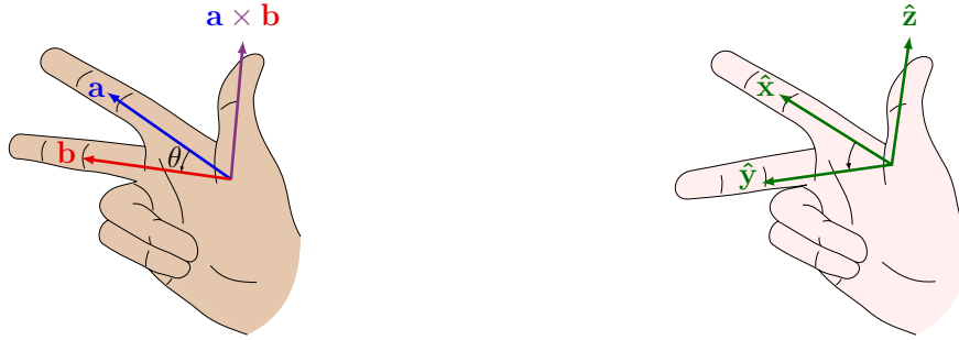
(a) The right-hand rule gives the direction of the vector product. (b) Conventionally, we use a right-handed coordinate system.
