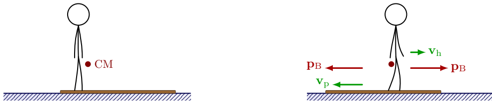
(a) Before: Brian and the plank are at rest. The total momentum is zero. (b) After: Brian starts walking, and the plank “recoils”. The total momentum is still zero.
