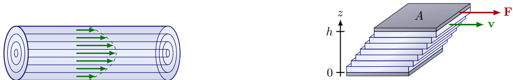
(a) Pipe with laminar flow: Layer close to the wall go slower due to drag forces. The dashed line is the laminar boundary layer .
