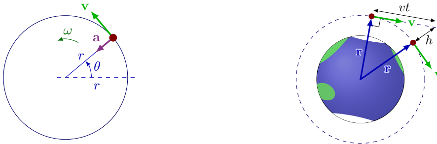
(a) A constant centripetal acceleration is perpendicular to the velocity and changes its direction.
