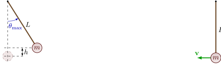
(a) Pendulum released from rest at an angle \theta_{\max} . (b) Pendulum has the maximum speed at \theta = 0 .
