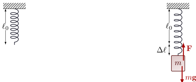
(a) Without a mass, the spring has length \ell_0 . (b) Elongation \Delta\ell due to gravity.
