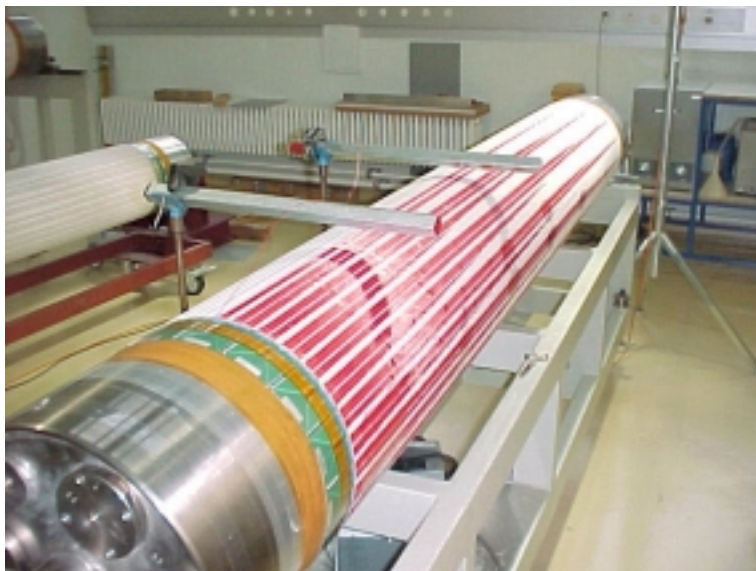
Figure 7.1: Construction of the cathode plane for the innermost chamber of CIP on the steel mandrils. Seen here are the flange at the -z end from which the coaxial cables fan out to the approximately 1500 cathode pads. The cables are embedded into a Rohacell cylinder.
