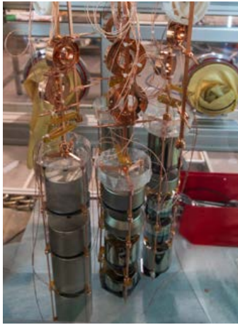
Figure 4.4: Left: four detector strings deployed as part of the PGT. Right: ^{228}\text{Th} calibration spectra acquired during the PGT.
