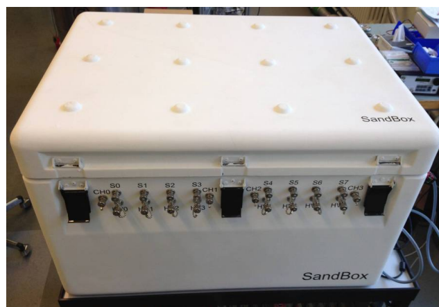
Figure B.5: Sandbox, the light-tight black box PMT testing facility.
