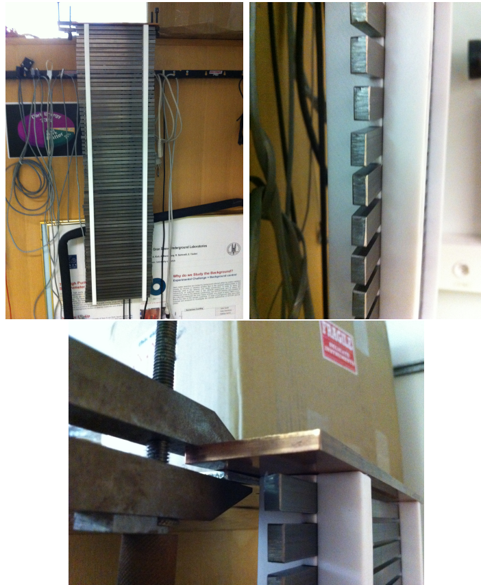
Figure 3.25: Overall view of the experimental setup to test the field cage segment
