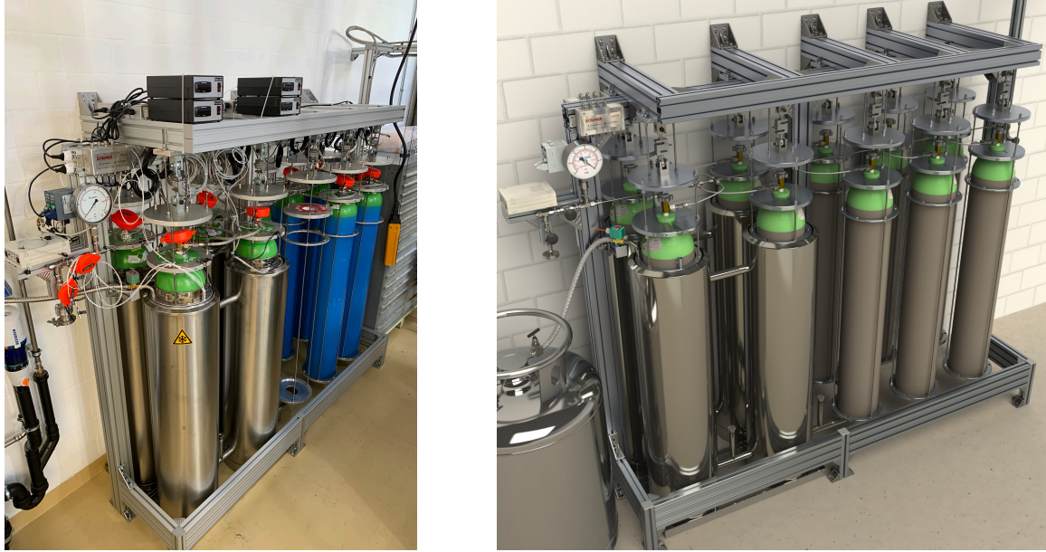
Figure 7.11: Gas xenon recovery and storage system of Xenoscope. Ten aluminium gas cylinders are suspended from load cells for mass determination, four of which are placed inside an inter-connected Dewar flask assembly. Left: Photograph with nine gas cylinders installed. Right: Rendering.
