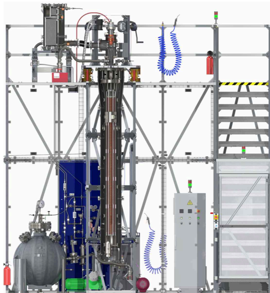
Test e - drift over 2.6 m (purification, high-voltage): U. Zurich
