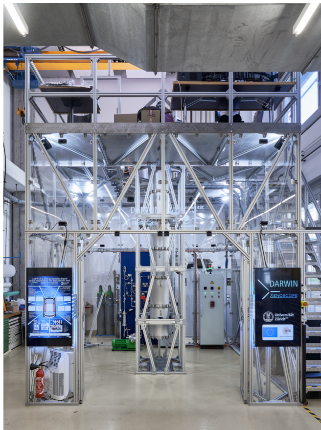
Test e - drift over 2.6 m (purification, high-voltage): U. Zurich
