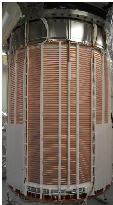
Figure 5.10: The TPC in its final place. The last PTFE protection panel is not yet installed and two of the cable trays and the PTFE insulator for the cathode connection are visible.
