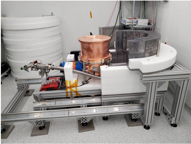
The dismantled prototype DAMIC-M experiment, showing layers of polyethylene, lead, and copper shielding. The CCDs are housed in the copper cryostat, with some components produced by UZH.
