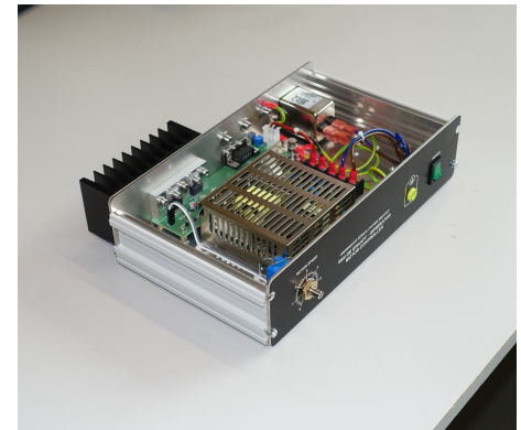
Left: 6-channel solar-powered battery charge controller for a potential mini-satellite application. This was the final practical work of the apprentice Lorena Mastroberti. Middle: frontend board for DAMIC-M. Right: Drivers for the Van De Graaff generators used in a lecture hall experiment. Load changes, which are caused by the charge shifts, can be visualized directly by the motor speed.
