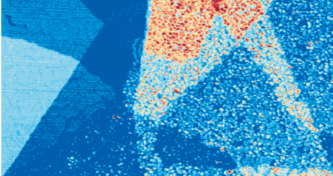
Tunneling microscopy image of a multilayer boron nitride on a platinum surface. 90 \times 180 \text{ nm}^2 (Data HY. Cun)
