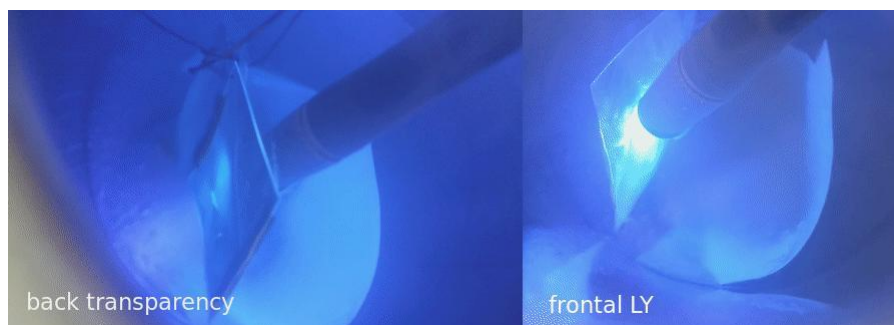
Figure C.4: ESR (adh) sample immersed in LN. The left image shows the blue light emitted by PEN which comes through the ESR reflector (back transparency). The image on the right shows the LY from the sample (frontal LY).
