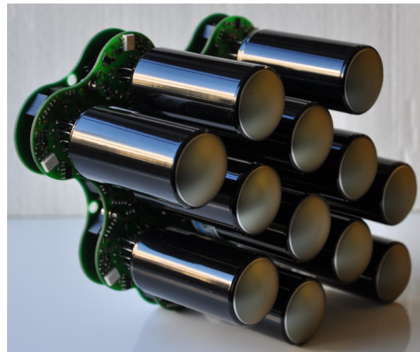
FIG. 6.4 – Assembled twelve-pixel group of the FlashCam photon detection plane.
