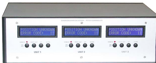
FIG. 18.7 – Motor control unit (front view).
