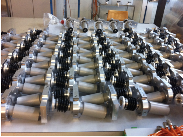
FIG. 6.2 – AMCs during mass production at UZH, to be used in the full Medium-size Telescope CTA prototype.
