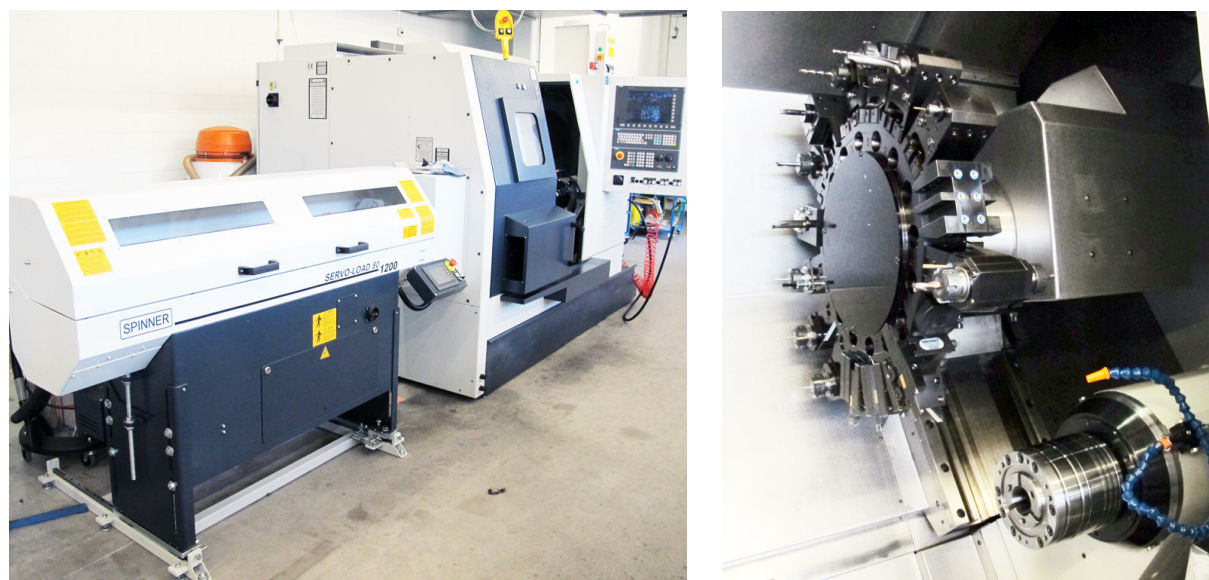
FIG. 17.1 – Left: new twin turret-turning center with bar loading system. Right: the turret for up to 16 tools and the right spindle.
