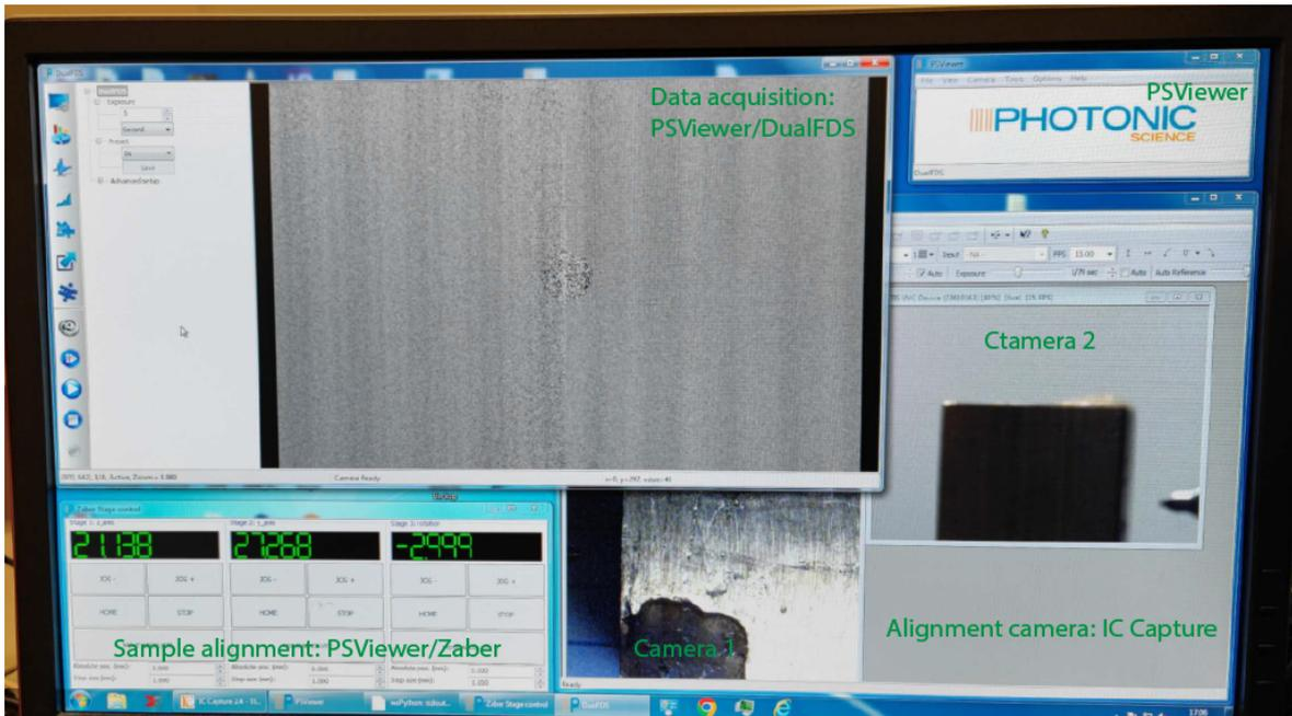
Figure 5: Data acquisition software (PSViewer) and alignment camera (IC Capture). Sample alignment is assisted by two motorized translational and one rotational degrees of freedom of the sample stage which is controlled under PSViewer/Tools/Zaber. Data acquisition is accessed under PSViewer/Camera/DualFDS, image can be exported under PSViewer/File.
